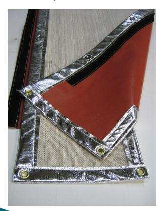
All parts to be custom fabricated using our extremely heavy duty ~96oz/yd<sup>2</sup> silicone coated glass designed to shed molten metal splash at 3000°F, all high temperature construction, grommets or 1/4 turn fasteners spaced on center along O.A.L to allow for easy installation/ removal, with flame retardant hook and loop along OAL, additional grommets on each loop end for "hanging" purposes.
