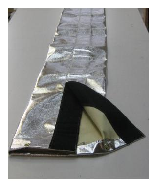
All parts are custom fabricated using our .042" thick Eko-Therm™ aluminized Kevlar® Blanket (shiny side out), all high temperature construction, grommets or ¼ turn fasteners spaced on center along O.A.L to allow for easy installation/removal, with flame retardant hook and loop along OAL, additional grommets on each loop end for "hanging" purposes.
