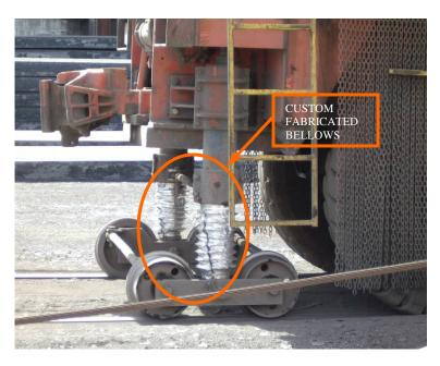
specialized heat resistant zipper closure to allow for easy removal for maintenance. The relatively minor cost of installing this custom fabricated bellows saves the steel plant thousands of dollars in maintenance costs!
